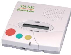
One touch of a button on the Base Unit links to our 24/7 Response Centre, where our trained staff will communicate with you through the two way speech facility and summon help if necessary. The unit is easily installed and links into your current phone line or broadband connection.
