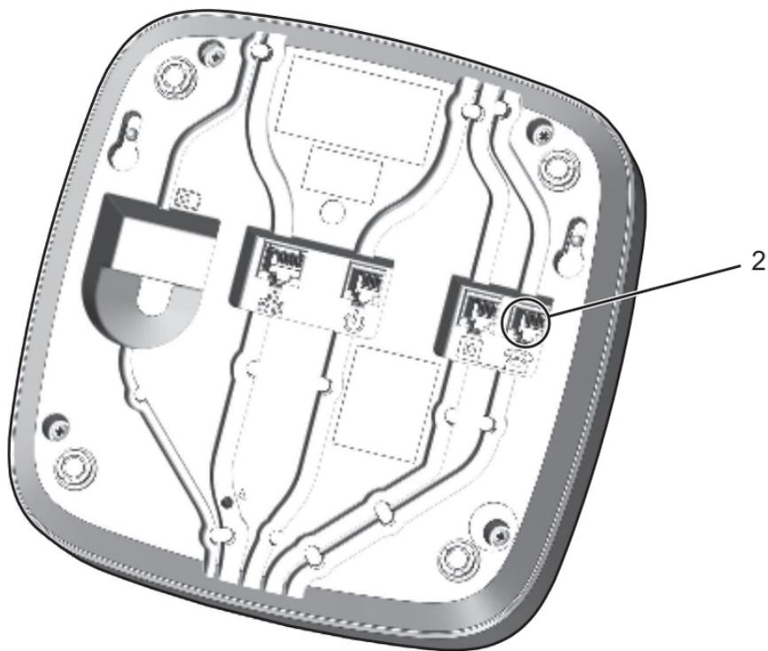
1. Insert the plug of the external telephone cable into the socket **(2)** on the TA74. Feed the cord through the cable channel and through the opening on the back of the unit.
