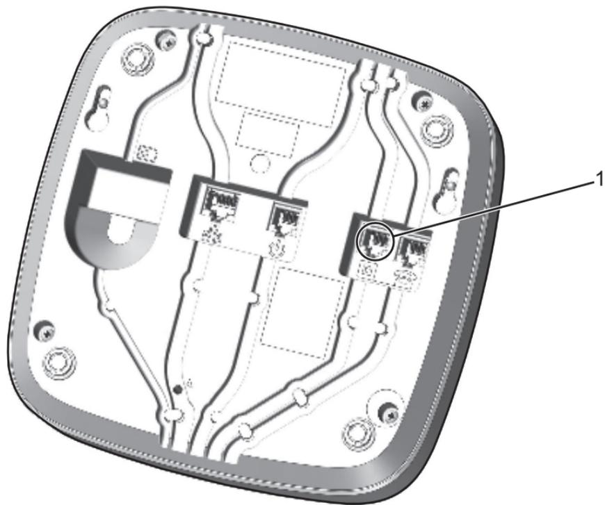
1. Insert the plug of the telephone cable into the socket **(1)** on the TA74. Feed the cord through the cable channel and through the opening on the back of the unit.
