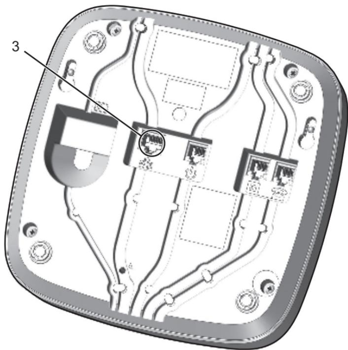
1. Insert the plug of the network connection cable into the socket **(3)** on the TA74. Feed the cord through the cable channel and through the opening on the back of the unit.
