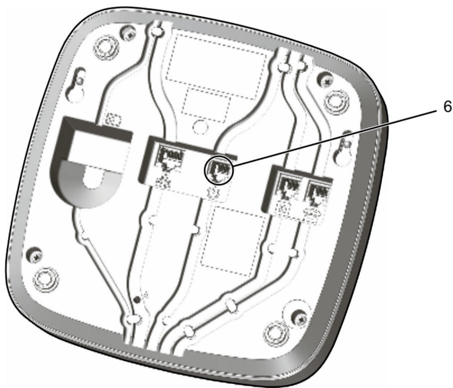
1. Insert the plug of the power adapter into the socket **(6)** on the TA74. Feed the cord through the cable channel and through the opening on the back of the unit.
